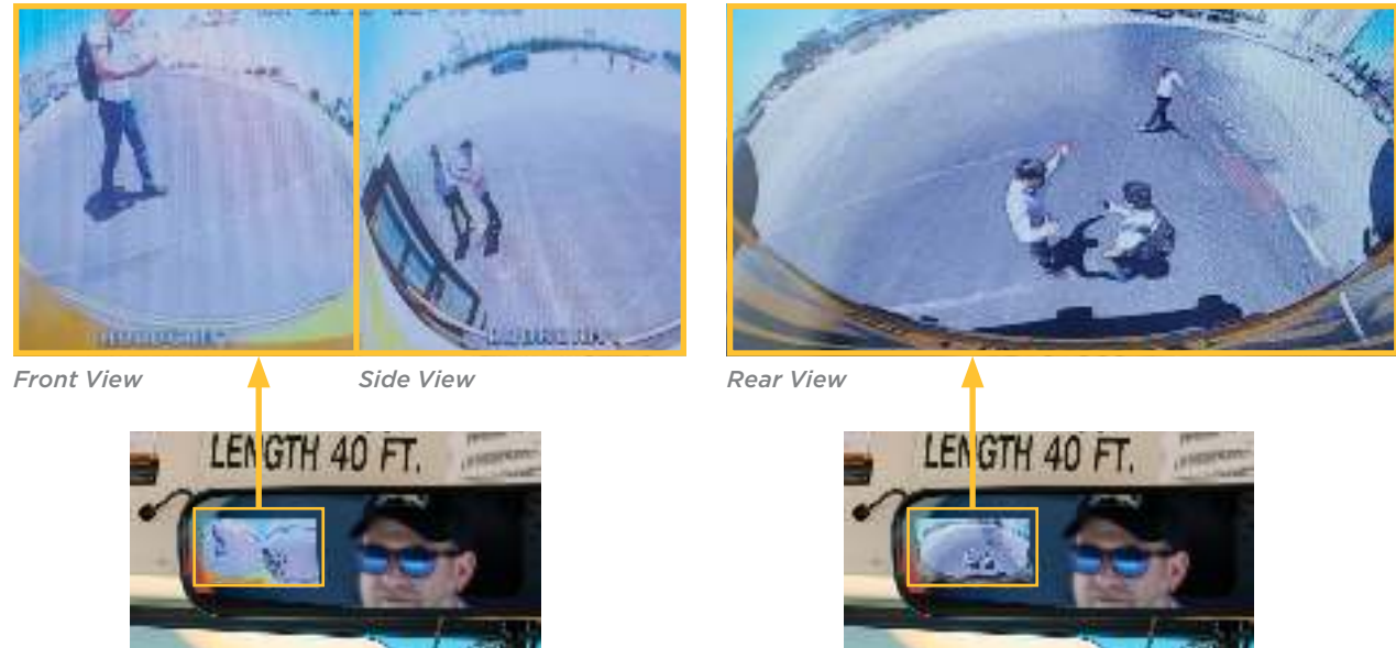
The Full View Camera System displays the most appropriate view based on the situation at hand, including backing up, opening the door, or the view of the front, side or rear of the bus.
