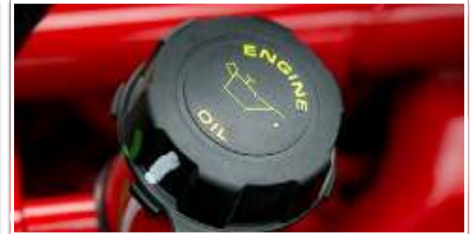
Routine service points are clearly labeled and easily accessed under the hood
