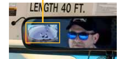
The Full View Camera System displays the most appropriate view based on the situation at hand, including backing up, opening the door, or the view of the front, side or rear of the bus.
