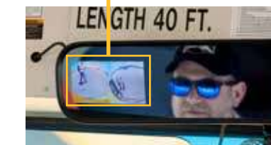
The Full View Camera System displays the most appropriate view based on the situation at hand, including backing up, opening the door, or the view of the front, side or rear of the bus.
